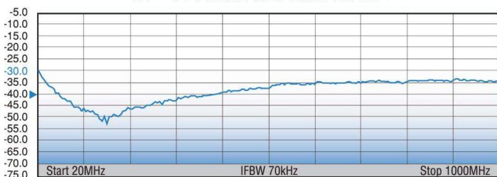
S11 TYPICAL RETURN LOSS (dB)
